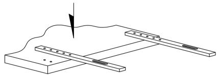
Align support board fixing holes over headboard fixing holes according to your desired height.
