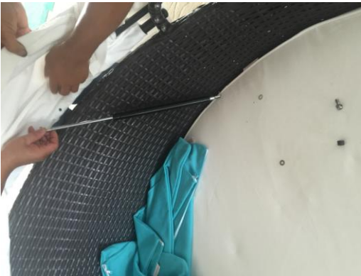
6.install the air bolt pole,use the screw to fixed the fabric and aluminum(the have a hole in the fabric and aluminum)
