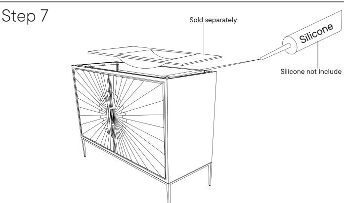
Apply a thin bead of silicone compound around the vanity base and set the vanity top carefully in place. Remove any axcess silicone compound with a wet rag.
