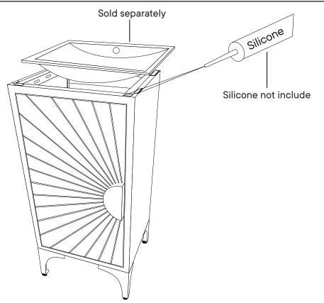
Apply a thin bead of silicone compound around the vanity base and set the vanity top carefully in place. Remove any axcess silicone compound with a wet rag.
