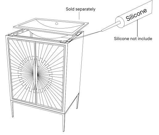
Apply a thin bead of silicone compound around the vanity base and set the vanity top carefully in place. Remove any axcess silicone compound with a wet rag.
