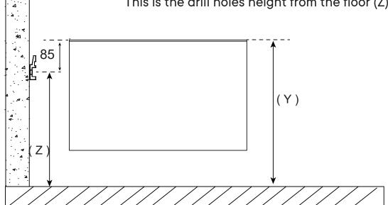
Please use minimum 2 holes on each group of the Medium Bracket and Long Bracket, and minimum 1 hole, to apply the wall plug and screw. Use additional holes when necessary.
