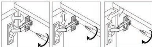
Adjust laterally    Adjust height    Adjust depth
