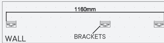
**15.4** Ensure your bracket measurements are correct before moving on to attaching the cabinet to the wall.
