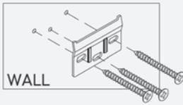
**15.3** Install bracket with 3 screws.
