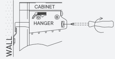
**15.8** Fasten the hanger's latch with the screw.
