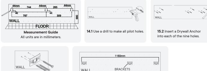
15.3 Install bracket with 3 screws. Repeat with other brackets.
