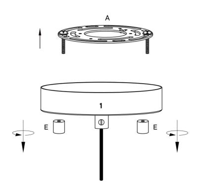
Determine your desired total drop of the Lamp Cord (2). Total drop is the distance from the ceiling to where you would like the bottom of the pendant to hang. Once decided, remove the screw on the Lock Sleeve (F) by using slotted head screwdriver, to adjust the height of hanging, secure the Lock Sleeve (F) at the Ceiling Canopy (1) by using slotted head screwdriver.
