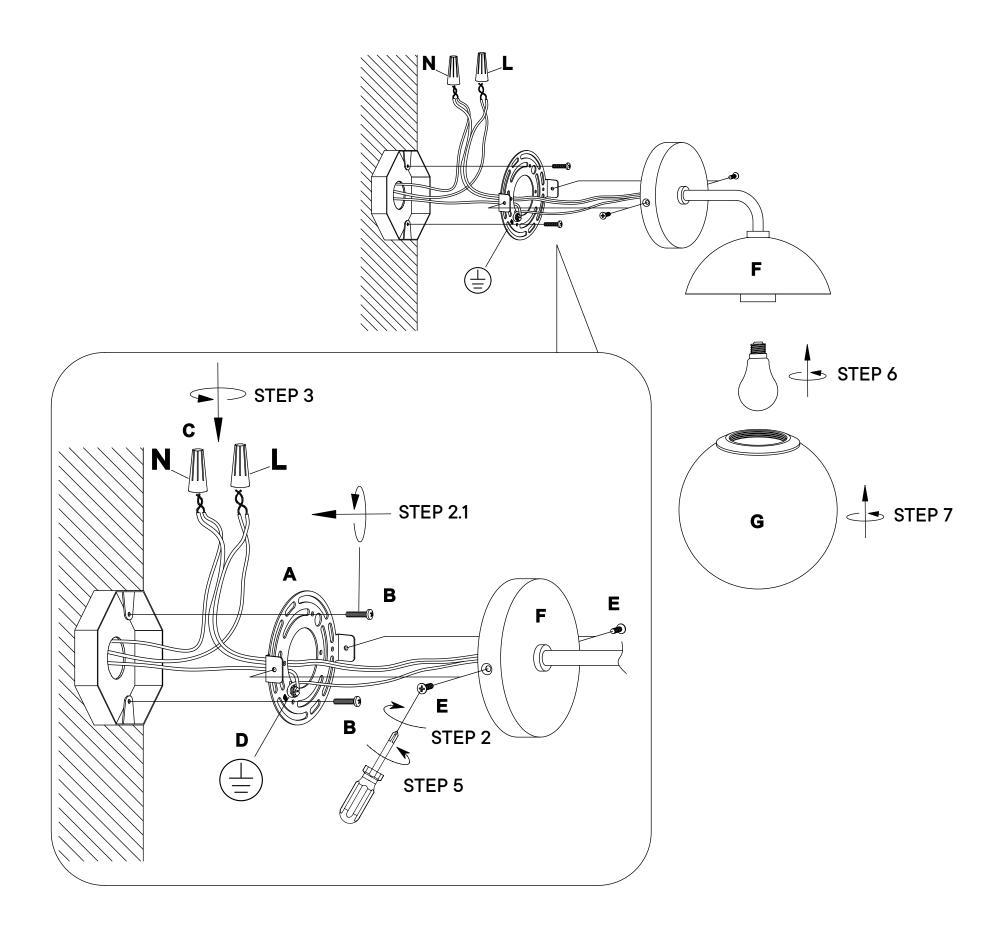
Before beginning **TURN OFF POWER** to the light from the fuse or circuit breaker.
