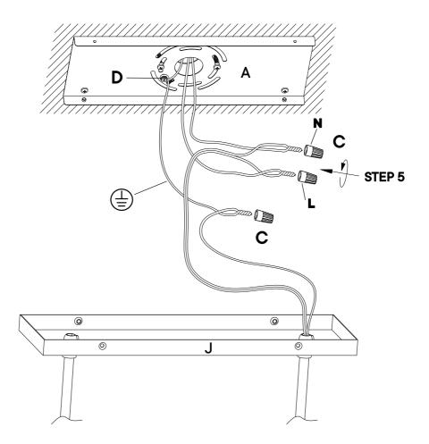
Continue to support fixture. Make sure all connected wires are carefully placed inside of box and canopy.
