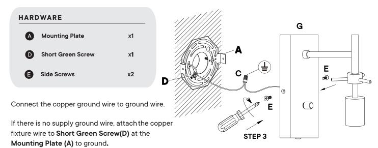
Attach the Lamp Wall Base (G) to the Mounting Plate (A) and secure with Side Screw (E)
