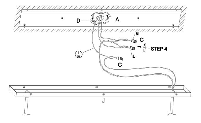
Continue to support fixture. Make sure all connected wires are carefully placed inside of box and canopy.
