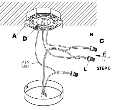
Continue to support fixture. Make sure all connected wires are carefully placed inside of box and canopy.
