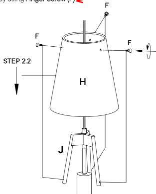
Determine your desired total drop of the lamp. The total drop is the distance from the ceiling to where you would like the bottom of the pendant to hang. You may use all rods or the combination of the rod to get your desired lamp height. Once decided, tighten the rod/tube accordingly.
