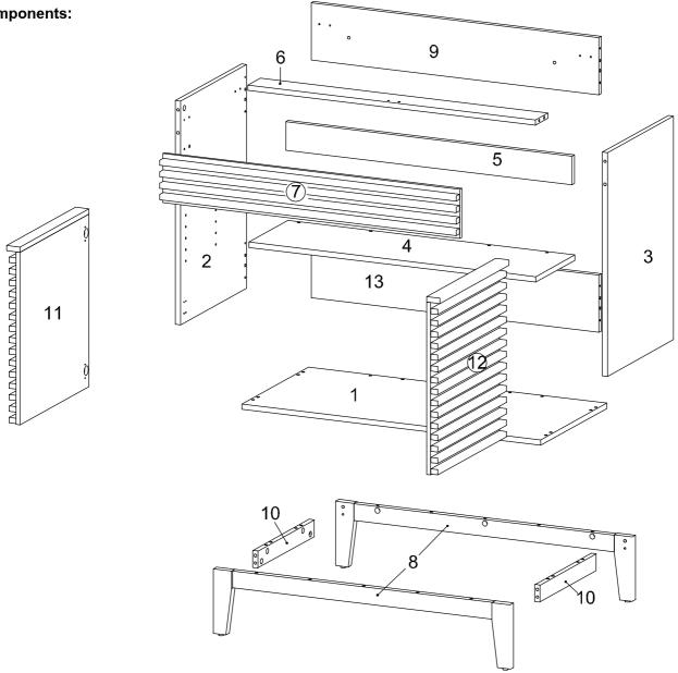
**Bottom Board** 2 Side Board Left Side Board Right 1 x1 **x**1 3 **x**1 Adjustable Shelf 5 Support Board 1 Support Board 2 4 6 **x**1 **x**1 х1 8 Assembly Leg Back Board 1 7 Front Skirt x1 x2 9 **x**1 Frame Door Right x1 Support Leg 10 x2 11 Frame Door Left x1 12
