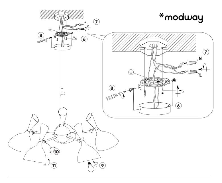
**Step 6** Attach the **Mounting Plate (A)** to the junction box in the ceiling and secure it with **2 Long Screws (B)**.
