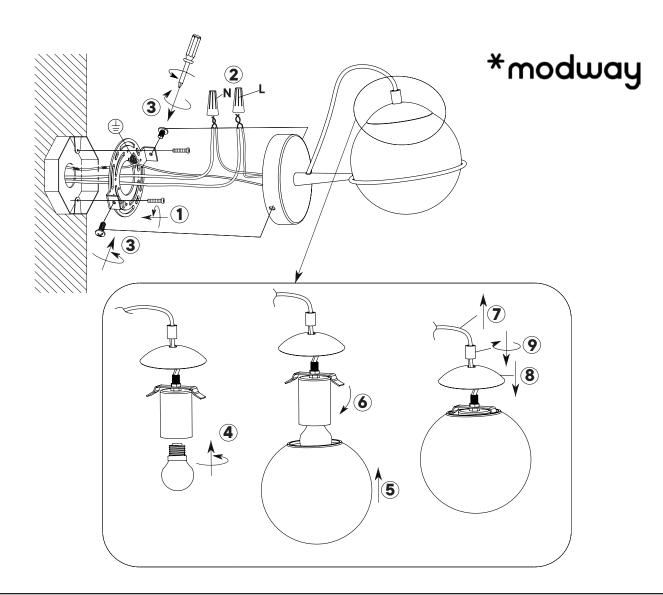
**Step 1** Attach the **Mounting Plate (A)** to the junction box in the wall and affix it with **2 Long Screws (B)**.
