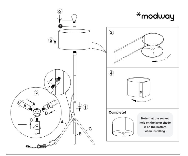
**Step 1** Connect the lower center pole to the upper center pole.
