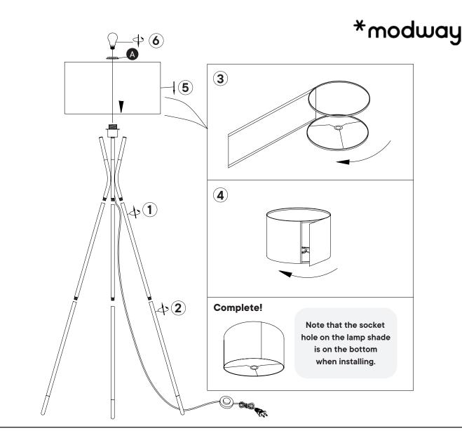
**Step 1** Connect the middle metal tubes to the upper metal tubes.
