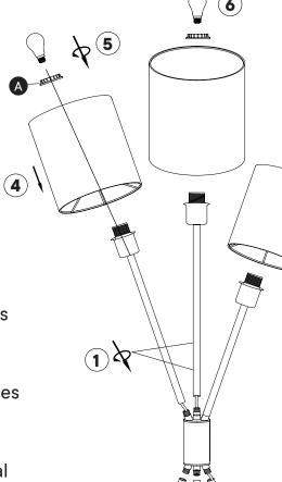
**Step 1** Connect the upper metal tubes to the center housing.
