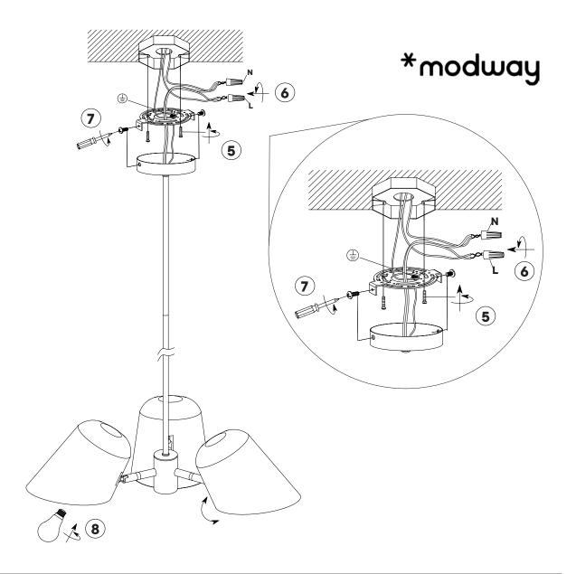
Step 5 Attach the Mounting Plate (A) to the junction box in the ceiling and secure it with 2 Long Screws (B).
