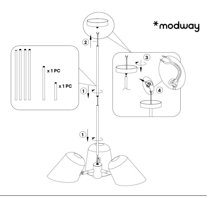
**Step 1** Position the three lamp shades as shown in the drawing. Pull the wire through the metal rods and connect the metal rods to the center housing of the chandelier.
