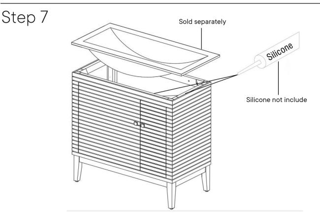
Apply a thin bead of silicone compound around the vanity base and set the vanity top carefully in place. Remove any axcess silicone compound with a wet rag.
