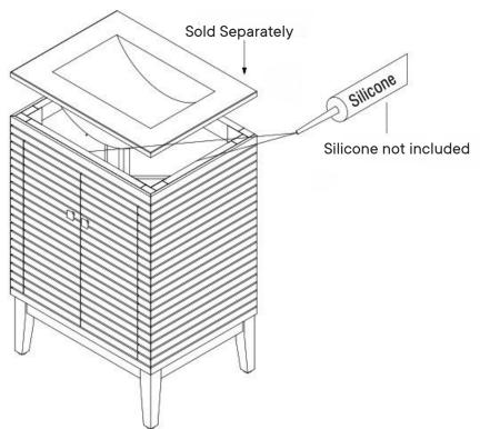
Apply a thin bead of silicone compound around the vanity base and set the vanity top carefully in place. Remove any axcess silicone compound with a wet rag.
