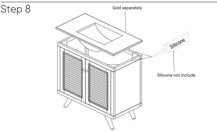
Apply a thin bead of silicone compound around the vanity base and set the vanity top carefully in place. Remove any axcess silicone compound with a wet rag.
