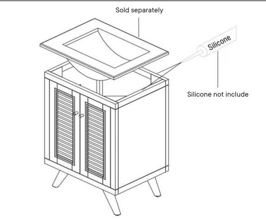
Apply a thin bead of silicone compound around the vanity base and set the vanity top carefully in place. Remove any axcess silicone compound with a wet rag.
