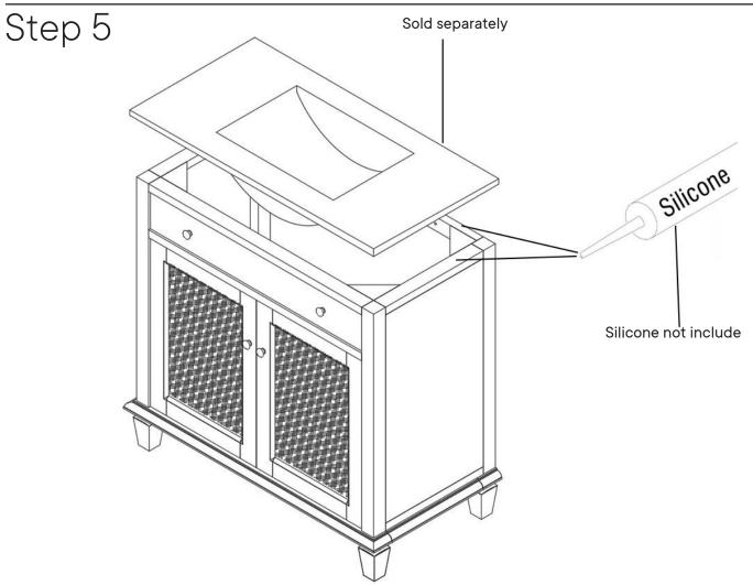
Apply a thin bead of silicone compound around the vanity base and set the vanity top carefully in place. Remove any axcess silicone compound with a wet rag.
