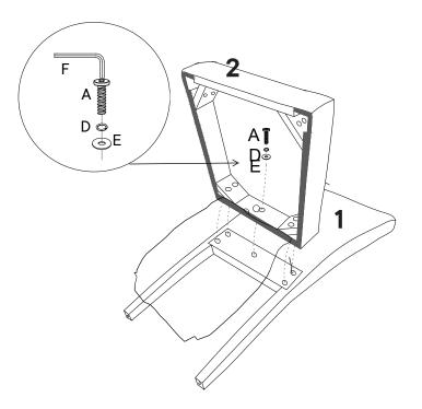
NOTE : Do not fully tighten the bolt
